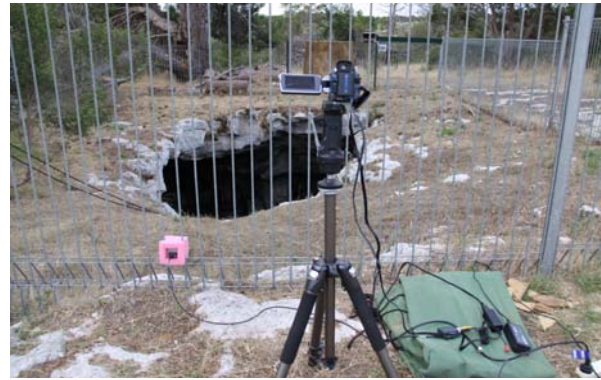
The thermal imaging camera attached to the fence and the mini DV video recorder on the tripod showing how the equipment is set up.
